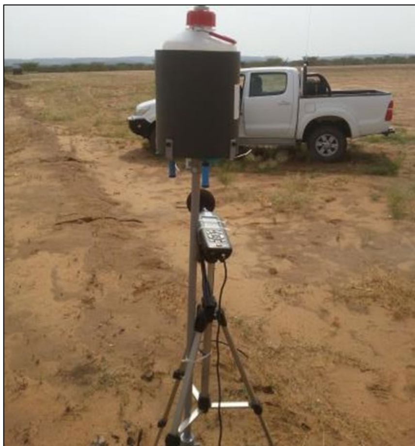
Figure 6.5-2: Deposited Dust Gauge, Diffusion Tubes and Noise Equipment Set Up for Data Collection at Amosing
