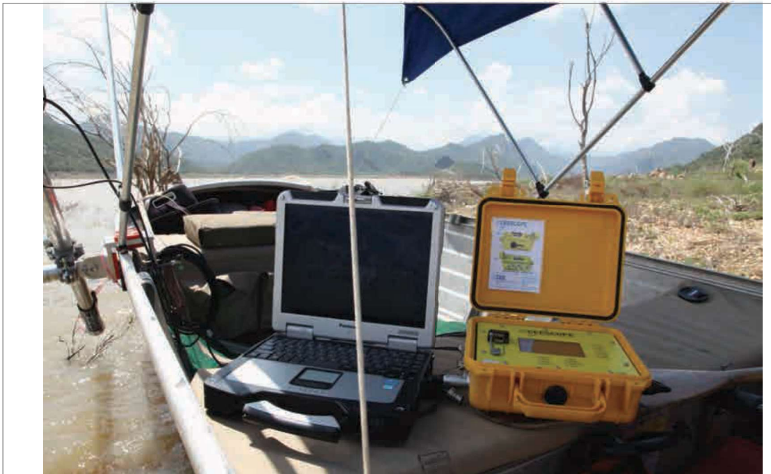
Figure 48: Boat-clamped transducer / GPS pole, laptop and CEESCOPE Control Unit
