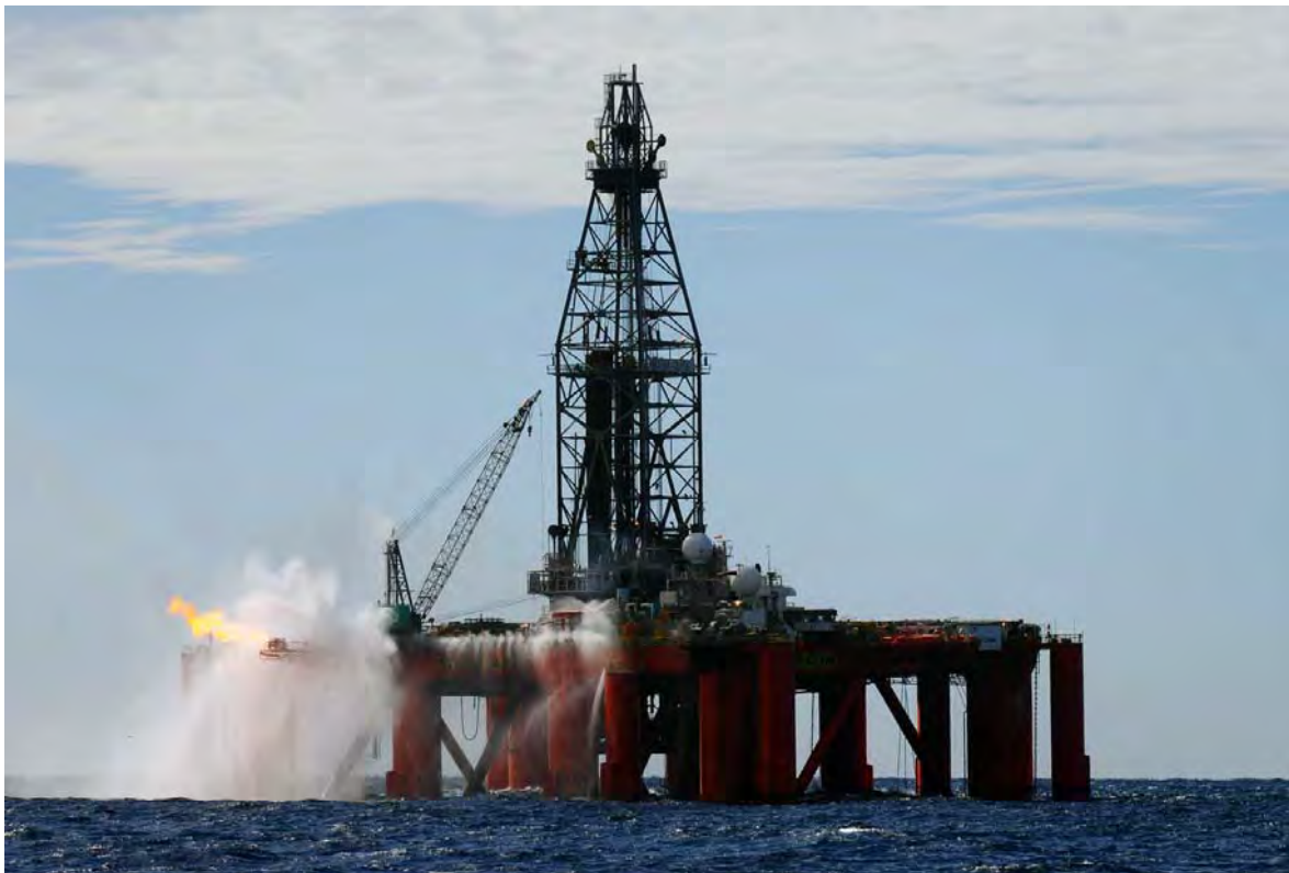
Figure 3.14 Well Testing on a Semi-Submersible MODU
