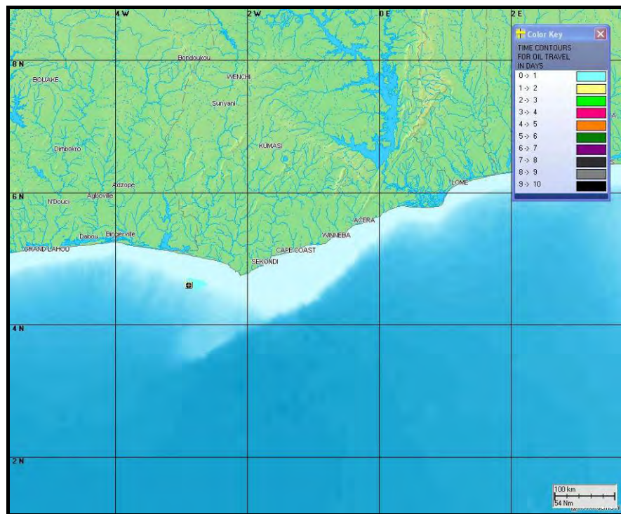
Figure 12. Marine gasoil spill of 10 Tonnes at the FPSO, a) water surface probabilities of oiling; b) travel time contours.
