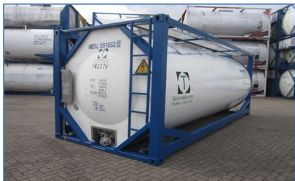
Figure 4-2: Typical ISO tanktainer
