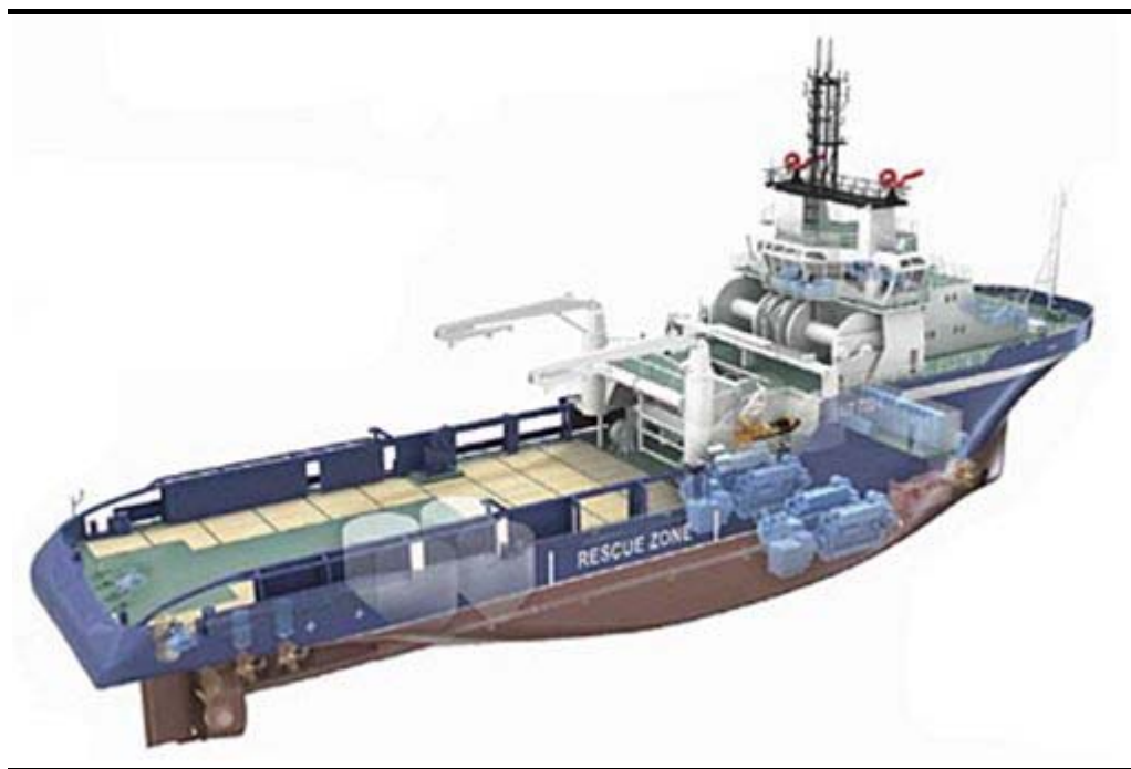
Figure 3.30 Typical MSV (80m length, 3160 gross tonnage and 180 tonnes bollard pull)
