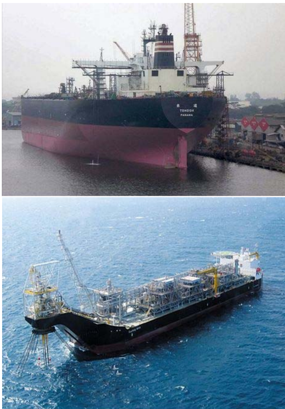
Figure 3.8 VLCC Tohdoh (top) Prior to Conversion to an FPSO Vessel (bottom)
