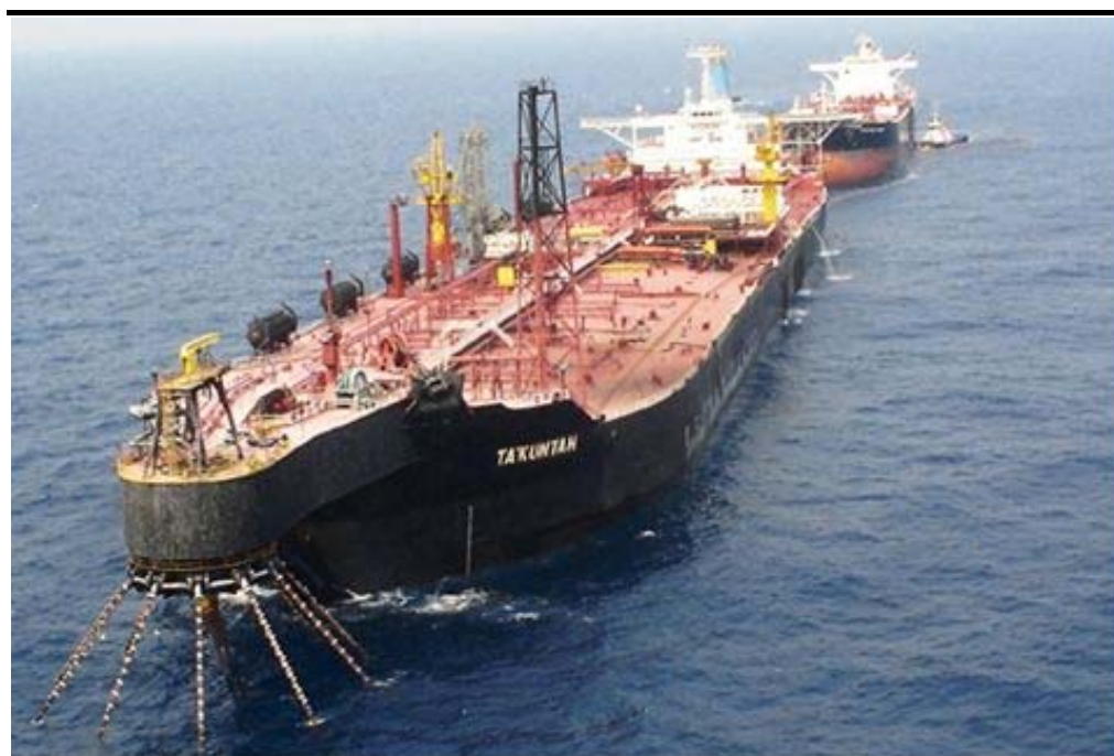
Figure 3.15 Typical External Turret Single Point Mooring System (on a FSU)
