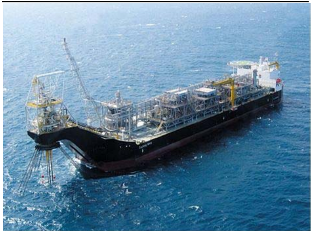
Figure 4.2 VLCC Conversion to a Turret Moored FPSO Vessel
