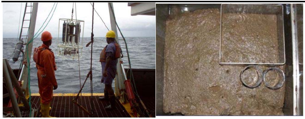
Figure 5.2 Water Sampler and Sub-sampling from Box Corer
