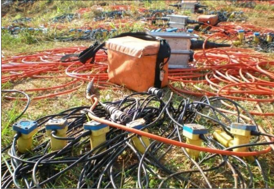
Plate 2.3: Geophones, batteries, cables and digitizing units before deployment on a seismic line.
