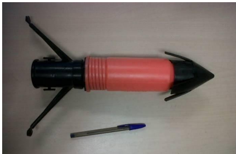
Plate 2.2: Dynamite charge (with plastic anchors) proposed as an alternative seismic source for the survey.
