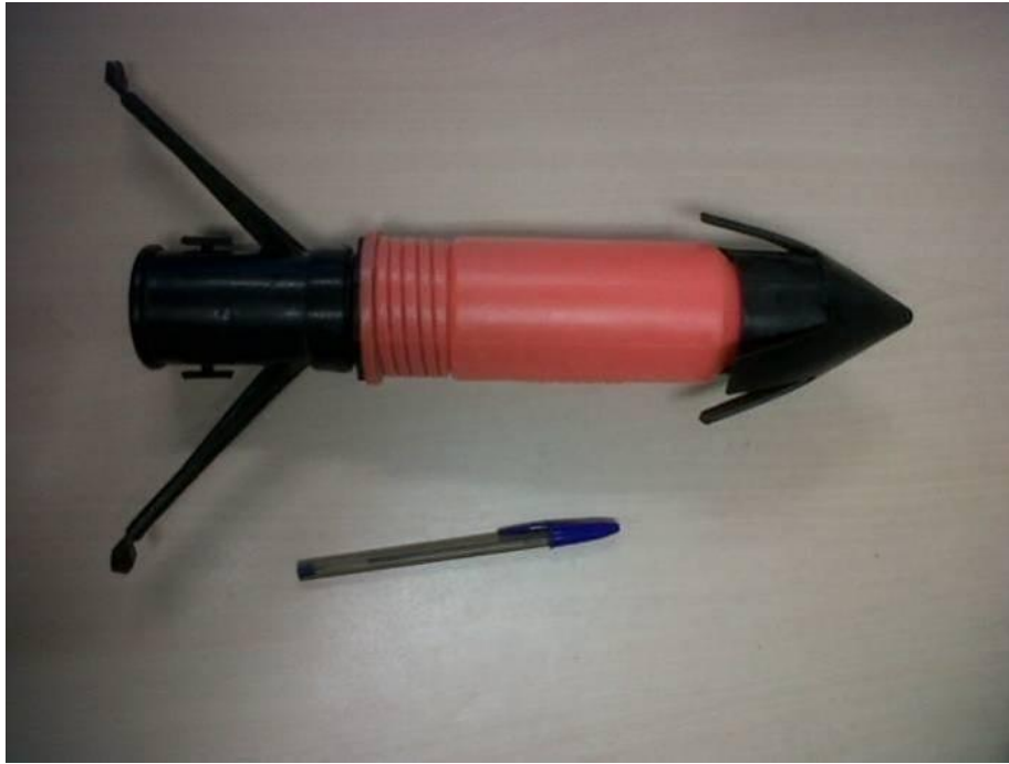
Plate 2.2: Dynamite charge (with plastic anchors) proposed as secondary acoustic source for the survey.
