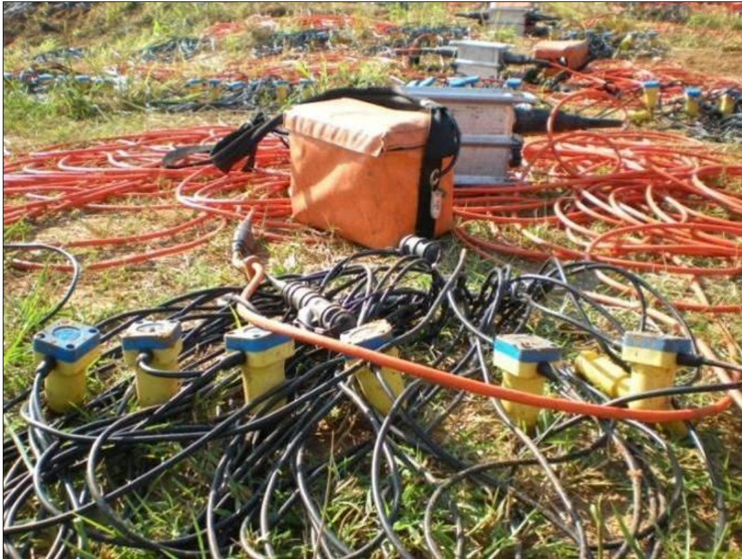
Plate 2.3: Geophones, batteries, cables and digitizing boxes before deployment on a seismic line
