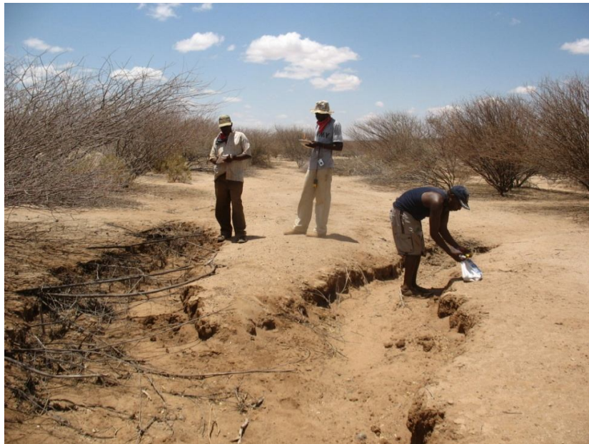
Plate 17: Mapping Unit PS2, mid of Gatab and Kargi. Note the gully forming due to the sodic nature of the soil
