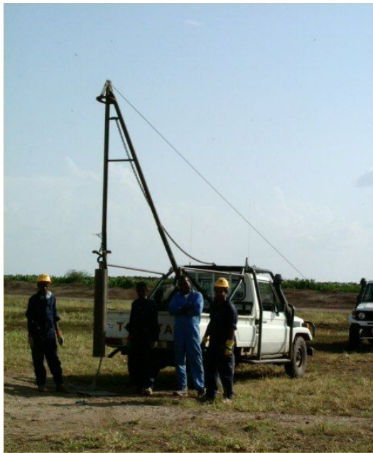
Plate 66: LVL weight drop unit
