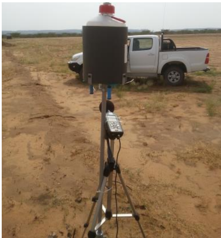
Figure 6-1: Deposited dust gauge, diffusion tubes and noise equipment set up for data gathering at Amosing 5
