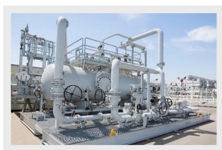
Typical production units to be installed on well pads
