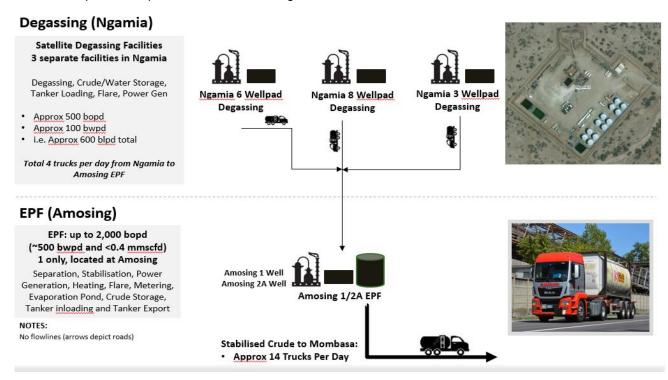
Figure 3: Summary Schematic of the EOPS Project including aerial image of Amosing-1 and articulated truck loaded with tanktainer (From Tullow EOPS ESIA Consultation Presentation)
