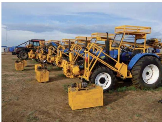
Tractor drilling rigs during seismic operations, Ethiopia.
