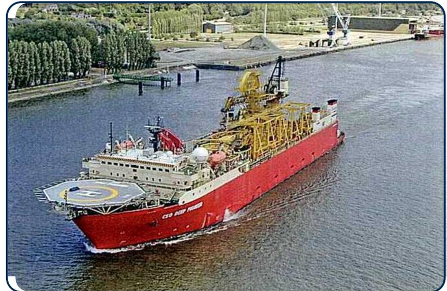
Subsea installation vessel; flexibles, risers, umbilicals
