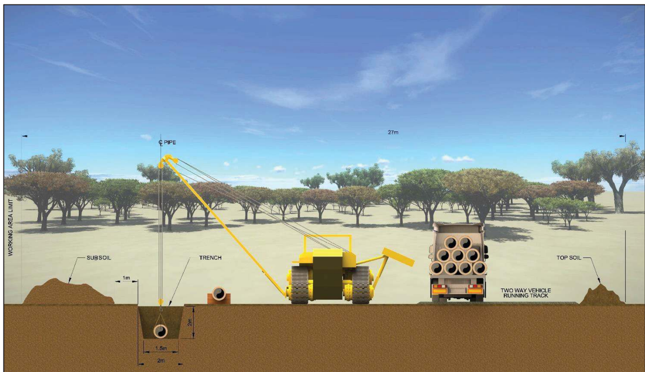
Figure 5.5-1: Indicative RoW for Water Pipeline Construction
