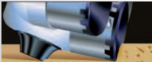
PDC (polycrystalline diamond compact) cutting
