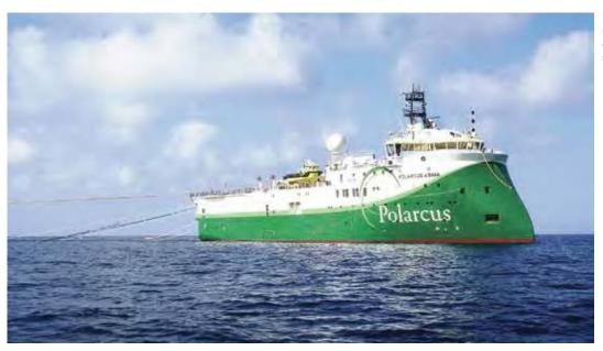
Left: Polarcus Asima seismic vessel, which carried out a 3D seismic survey, offshore Namibia.
