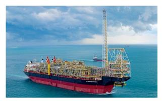
Tullow Ghana is operator for the Jubilee and TEN fields in Ghana, with two producing Floating Production Storage and Offloading (FPSO) Vessels: FPSO Kwame Nkrumah and FPSO John Evans Atta Mills. FPSOs are comparable to a chemical processing plant with tanker storage capabilities to process and store extracted hydrocarbons.
