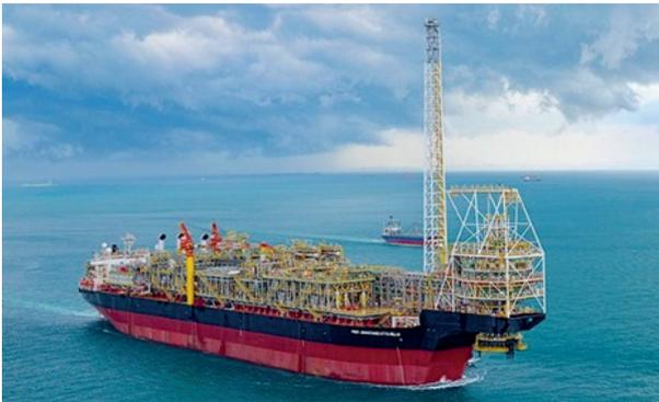
Tullow Ghana is operator for the Jubilee and TEN fields in Ghana, with two producing Floating Production Storage and Offloading (FPSO) Vessels: FPSO Kwame Nkrumah and FPSO John Evans Atta Mills. FPSOs are comparable to a chemical processing plant with tanker storage capabilities to process and store extracted hydrocarbons.
